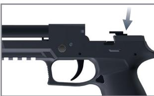
5. Lubricate the hammer with a small amount of silicone oil.
