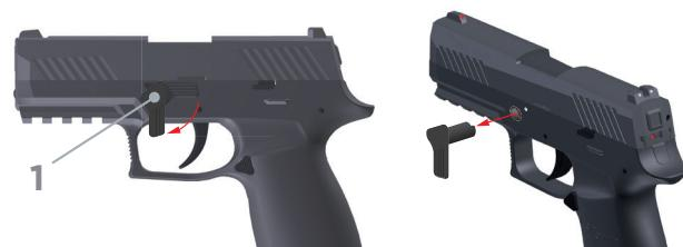
1. Swing the disassembly lever 1 downwards, then remove it from the gun.
