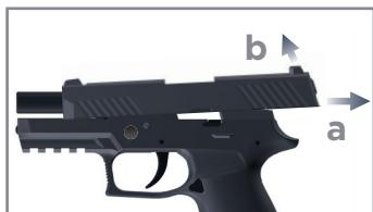
2. Pull the slide backwards (a) and upwards (b).
