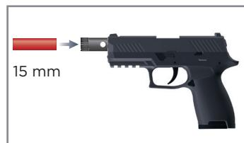
3. Insert the flare into the extra barrel, with the open end of the flare cartridge first.
