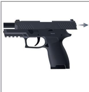
4. Pull the slide back until it stops and allow it to slide forward.
