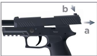
7. Pull the slide back completely (a) and push it downwards (b).
