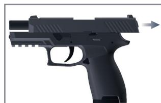
4. In order to load the first cartridge into the barrel, pull the slide back until it stops, then release the slide.
