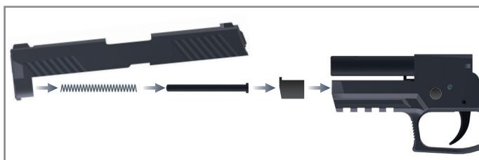
6. Then re-assemble the slide, the guide sleeve, the spring as well as the spring guiding rod in the order shown in the picture, and in the next step push the slide on the gun from the gun's front end.
