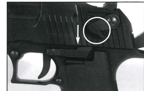
After emptying the magazine, push the safety mechanism back into the locked position.
