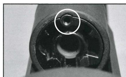
Push back the slide cover and ajust the bax system with an allen Key
