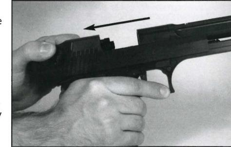
In order to fire, you have to cock the gun : pull the slide backward as shown and release.
